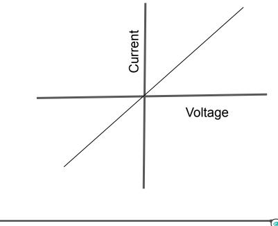
Yes, as the line has a constant gradient and passes through the origin. This shows that voltage is directly proportional to current
